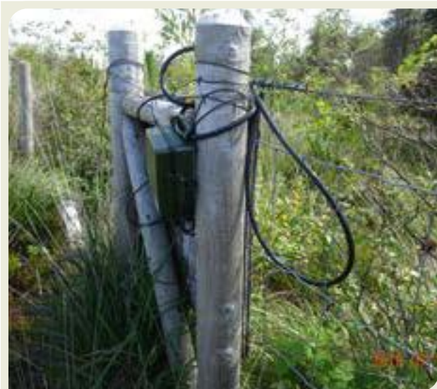
Plate 55a: Bat monitoring. Passive Bat recorder. (SM4 Passive Detector) deployed on fenceline close to wetland ponds on the wayleave
